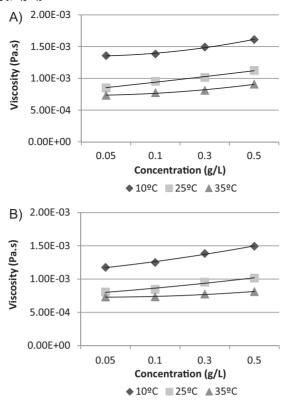
**Figure 2.** Viscosity behavior of the biopolymer produced by *Aureobasidium pullulans* IOC 3011 strain, using brewery residual yeast as nitrogen source at C/N ratio of 100 (A), and pullulan Sigma-Aldrich standard (B) at different concentrations in solution at a rate of shear of  $613\,\mathrm{s}^{-1}$  (Advanced Rheometer 2000, 10, 25 and 35 °C) [Initial viscosity of different media: approximately  $1.33\times10^{-3}\,\mathrm{Pa.s.}$  (Newtonian behavior)].
