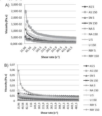
Figure 1. Viscometric profiles of different media compositions fermented with IOC 3467 (A) and IOC 3011 (B) strains [AS - ammonium sulfate, SN - sodium nitrate, AN - ammonium nitrate, U - urea; RBY - residual brewery yeast, carbon/ nitrogen 5 and 150; Advanced Rheometer 2000, 25  $^{\circ}$ C; initial viscosity of different media: approximately  $1.33 \times 10^{-3}$  Pa.s. (Newtonian behavior)].
